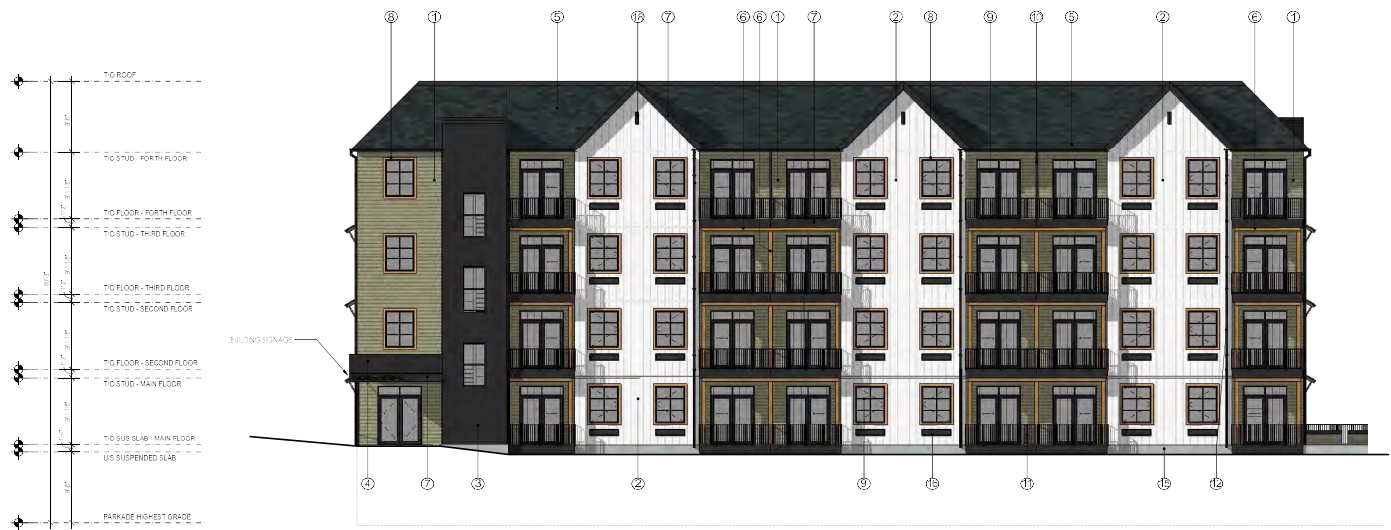
1 BUILDING A1 EAST (FRONT) ELEVATION 1/8" = 1'-0"
