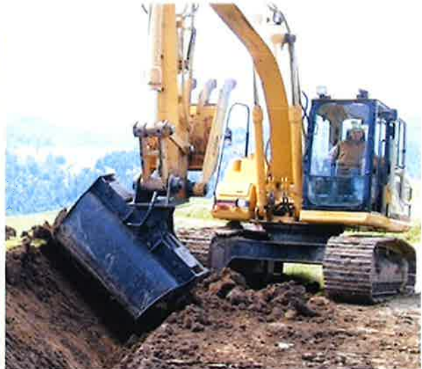
Excavator with tilt bucket
