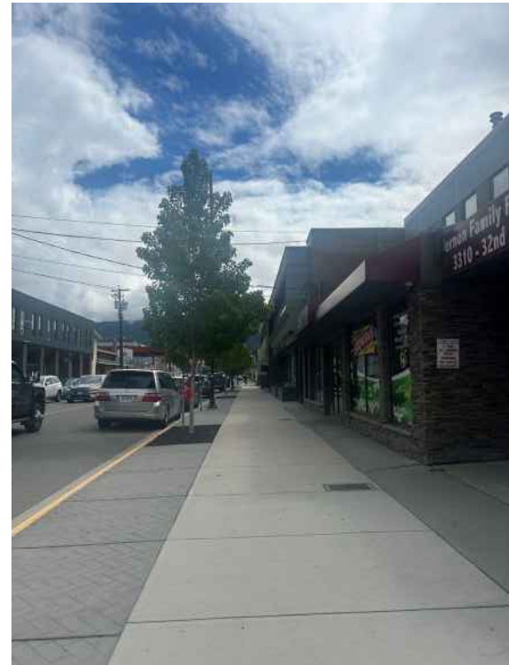
Grade-separated Concrete Sidewalks
